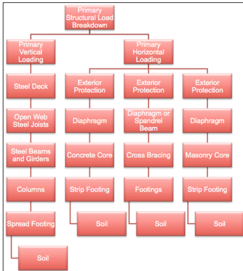
Figure 5.1.1 Primary Structure Load Breakdown
