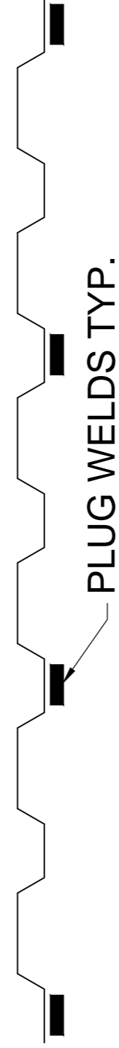
TYPICAL DIAPHRAGM CONNECTION 1:10 4 BUTTON WELDS BUTTON PUNCH 600c/c MAX.
